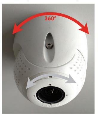
Axis 3: Rotating the sensor module in the PTMount
