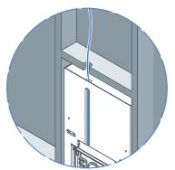
Ensure a clear path is maintained for cable insertion
