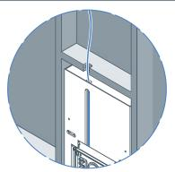
Ensure a clear path is maintained for cable insertion
