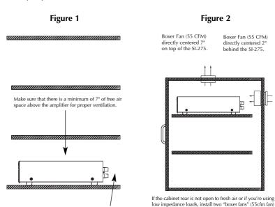
to provide continuous air flow into and out of the cabinet.
