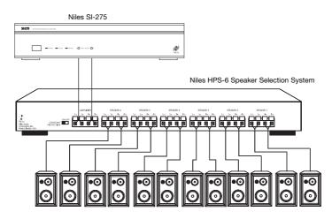
Speaker selection systems allow each pair of speakers to be turned on and off from your equipment location (or even via remote control).
