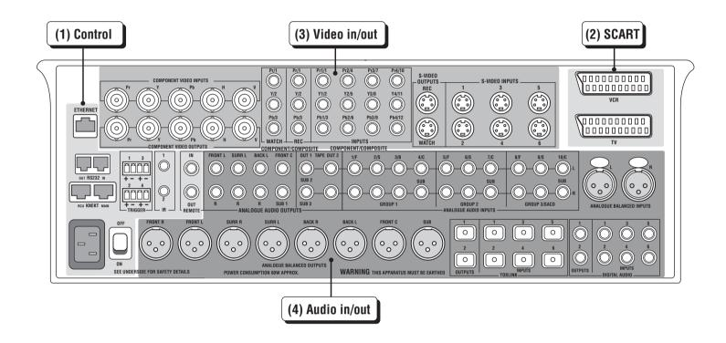
The diagram above shows the connectors available on the back panel of your KISTO. Connectors are arranged in named groups according to function. The connector groups and connection functions are listed in the manual in sections as shown on the diagram.
