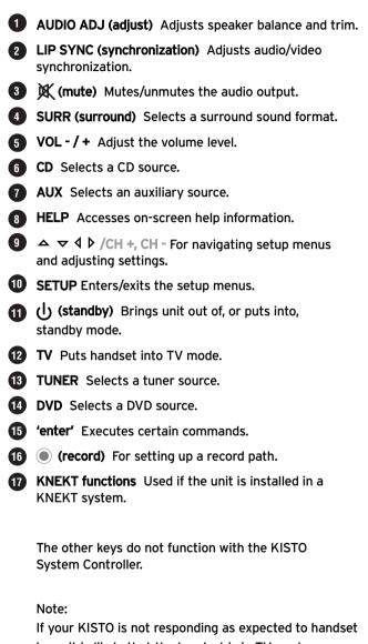
keys, it is likely that the handset is in TV mode. To correct this, press any of the source keys (DVD, CD, TUNER or AUX) on the handset.
