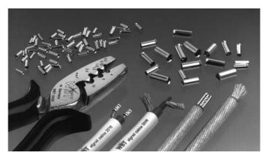
WBT offers a wide range of crimping accessories: gold-plated cable sleeves made of highly conductive electrolyte copper, E-Cu > 99.996% (in sizes from 0.5 to 16 mm²/22-5 AWG), sleeves made from fine silver (1.5 to 6 mm²/17-10 AWG), special crimping pliers for the above requirements and a complete crimping set for beginners. WBT-0403 crimping pliers/WBT-0411 crimping set.
